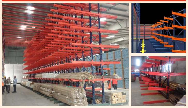
Customised racks for the storage of long sections, can be handled manually or by MHE. UNIQUE has commissioned up to G+7 cantilever racks.
