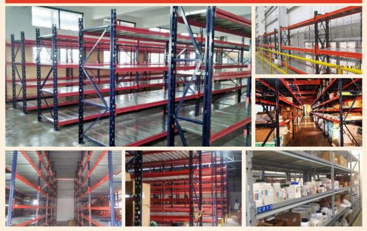
Light, Medium and heavy duty customised racks wherein handling of products is manual. Load carrying capacity is from 100 Kg - 2000 Kgs per level. It has excess to each and every items stored on racks.
