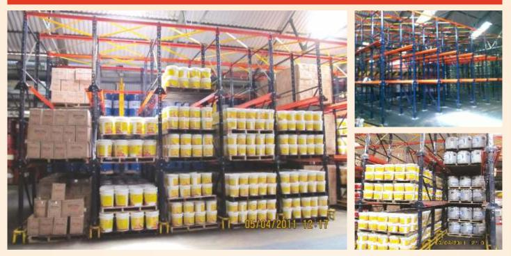
Customised racks with depth wise storage of pallets on cantilever runner beams. It works on LIFO principle only. It gives maximum utilization of space. UNIQUE has commissioned upto G+5 racks with 10 deep pallets.
