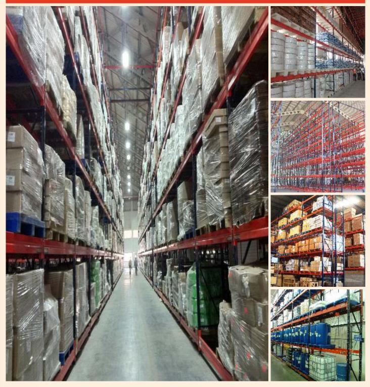
Heavy and Medium duty customised racks wherein Load is kept on the pallet which is handled by a MHE to utilize maximum available height. It allows the access to each and every pallet stored on racks.
