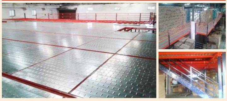
Customised, Self supported modular structure from formed sections with galvanised/ powder coated deck panels as flooring with provisions of staircase, lift, chute and railings. Standard load carrying capacity of the floor is 500 kgs/sq.m.
