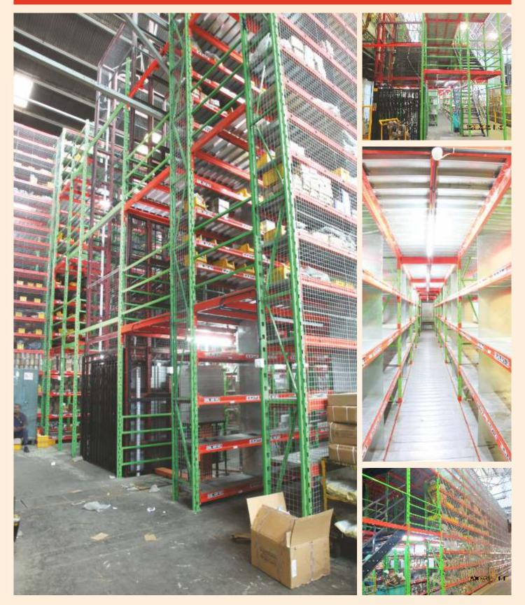
Heavy, medium and light duty customized shelving systems with a provision of catwalks/mezzanine at every 2.5m height to utilize heights available in the warehouse/store wherein person can go up by staircase and goods can be handled through goods lift/MHE/Trolleys. Span of racks can be max upto 3m
