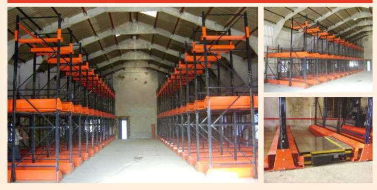
Customised racks with depthwise storage of pallets on cantilever runner beams with remote operated radio shuttle (pallet mover). It too works on LIFO and gives max utilization of space.
